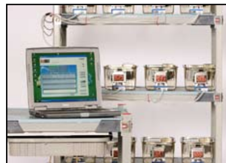
The BioDAQ electronics mount directly in place of the Unplugged adaptor plate.
